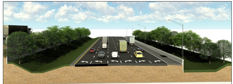
I-95 northbound exit ramp - Widening from 4 existing lanes to 6 proposed lanes
