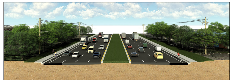
I-95 southbound exit ramp - Widening from 4 existing lanes to 6 proposed lanes
