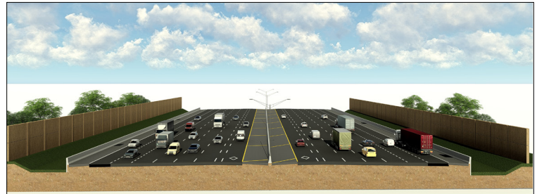
I-95 mainline - Adding an auxiliary lane on each side
